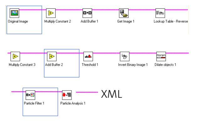
Figure 13 labview processing queue
