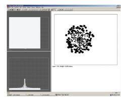
select the layer view [1] and go through the layers of the model [2], checking that there are no irregularities or incoherences (minor ones are not important). if this should be the case, re-export the project from the cad software and open it again in Zprint. it may be necessary to modify it before re-exporting it.
