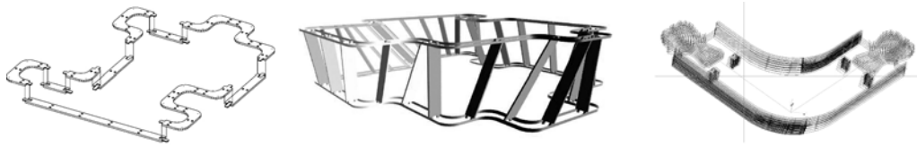
Figure 6. a) Alternating sequence of designed sections and intermediate segments generated by the plug-in; b) sequence of elements of a generated section calculated by Maya; c) milling paths in SurfCAM
