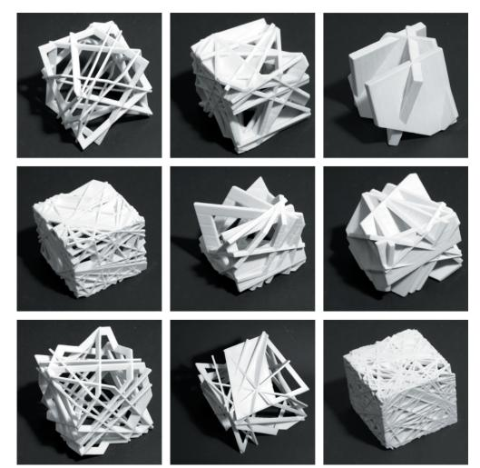
Figure 2. Examples of different cubes produced by a plaster 3D printer – showing different densities of the grid as well as a variety of possibilities offered by changing the frame thickness and proportions between the outside and inside cube.
